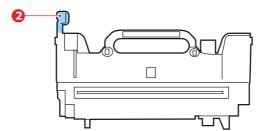
**9.** Lower the fuser into the MFP, locating the two lugs (3) into their slots in the metal partition which separates the fuser area from the image drums.
